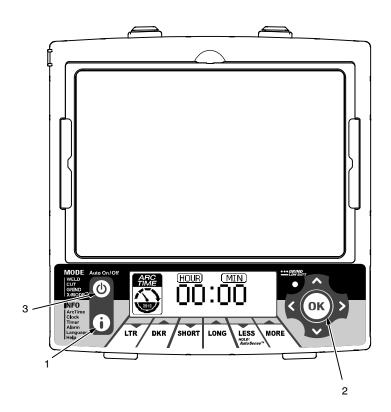
The arc time function records the amount of time the lens assembly is dark (exposed to an arc).
