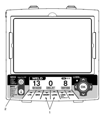
Lens Delay Adjustment Buttons
