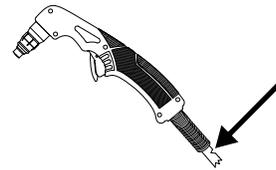
Inspect the torch lead. Replace if damaged.
