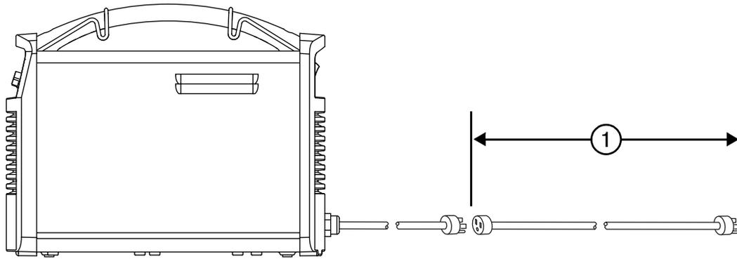
Use an extension cord of an appropriate wire gauge for the cord length and system voltage. Use a cord that meets national and local codes.
