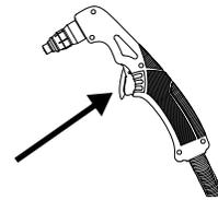
Inspect the trigger for damage. Inspect the torch body for cracks and exposed wires. Replace any damaged parts.
