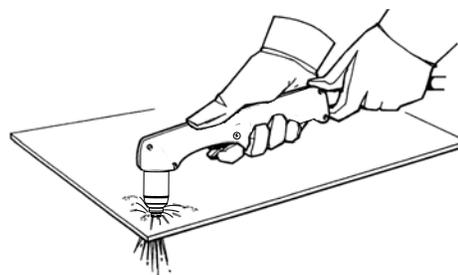
5. When the pierce is complete, drag the torch lightly along the workpiece to proceed with the cut.
