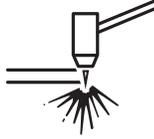
When cutting material up to 10 mm (3/8 inch) thick, start the torch at the edge of the workpiece to prolong consumable life.
