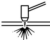
When cutting material up to 6 mm (1/4 inch) thick, use piercing to cut an interior feature. Piercing shortens the life of the deflector and the nozzle.
