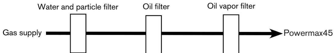
The filtering system should be installed between the quick-disconnect coupler and the power supply.
