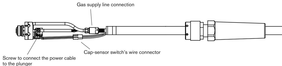
4. Use a #2 Phillips screwdriver and a 6 mm (1/4 inch) nut driver (or adjustable wrench) to remove the screw and nut that secure the torch's power cable to the plunger. (Turn the plunger if necessary to gain access to the screw.)
