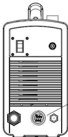
Receptacle for the remote-start pendant or a machine interface cable.
