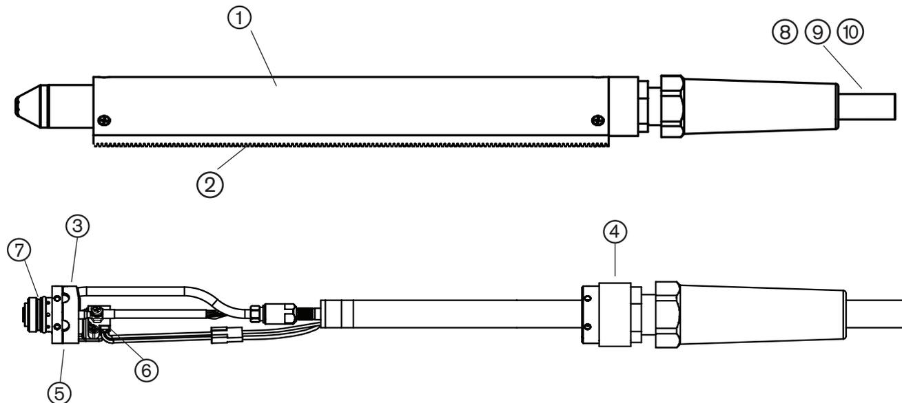
The entire machine torch and lead assembly can be replaced, or individual component parts can be replaced. Part numbers starting with 088 indicate complete torch and lead assemblies.
