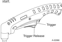
5. Bring the torch within transfer distance to the work. The main arc will transfer to the work, and the pilot arc will shut off.
