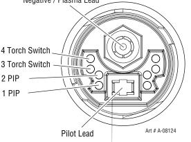
b) For machine torches using a remote pendant, Check continuity of Pendant switch circuit
