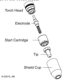
Torch Parts (Drag Shield Cap & Shield Cup Body Shown)
