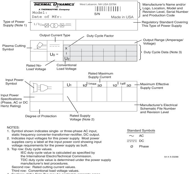
4. Sections of the Data Tag may be applied to separate areas of the power supply.
