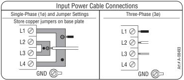
Single and Three Phase Input Power Wiring
