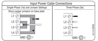
Single and Three Phase Input Power Wiring
