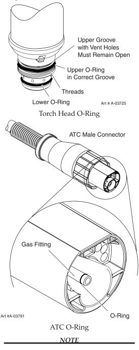
**DO NOT** use other lubricants or grease, they may not be designed to operate within high temperatures or may contain "unknown elements" that may react with the atmosphere. This reaction can leave contaminants inside the torch. Either of these conditions can lead to inconsistent performance or poor parts life.
