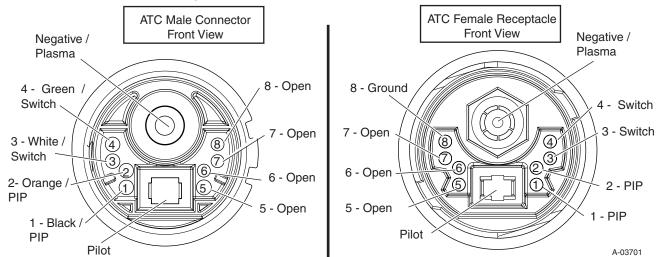
B. Mechanized (Machine) Torch Pin - Out Diagram
