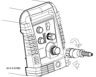
Connecting the Torch to the Power Supply 3. The system is ready for operation.
