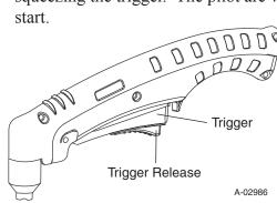
6. Bring the torch within transfer distance to the work. The main arc will transfer to the work, and the pilot arc will shut off.
