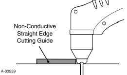
Using Drag Shield Cup With Straight Edge
