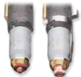
Note: Use the Ohmic Clip with the Shielded Tip design if ohmic plate sensing is required
