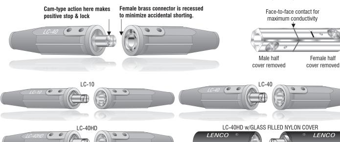
The glass filled nylon covers are designed for extreme heat and impact resistance applications.
