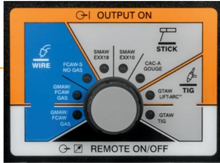
**LED process indicator.** Front panel process selections are illuminated with an LED that identifies the active process. This enables the selected weld process to be seen at a distance from the power source. Includes carbon arc gouging mode for enhanced arc stability and control, and two stick modes (EXX10 and EXX18) designed to reduce spatter and enhance arc starts.
