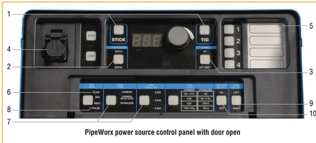
PipeWorx power source control panel with door open
