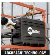
Make parameter changes at the weld joint, eliminating walks back and forth to the machine. Increase arc-on time and improve jobsite safety.
