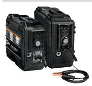
SuitCase® X-TREME™ 8VS951582SuitCase® X-TREME™ 12VS951543Lightweight, portable wire feeder for a variety of<br/>wires up to .062 inch. Holds up to an 8-inch<br/>(8VS) or 12-inch (12VS) spool of wire. Operates<br/>on open-circuit voltage eliminating the need for<br/>a control/power cord. See literature M/6.42.
