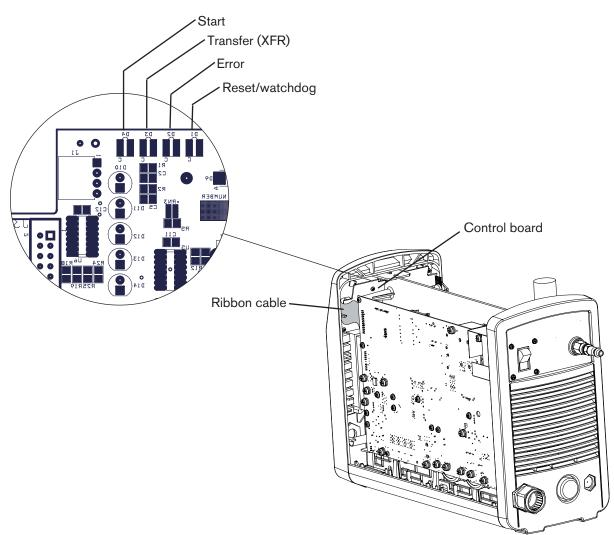
The control board LEDs are:
