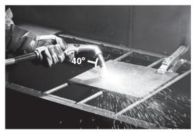
2. Hold the torch at a 40° angle with the nozzle about 1/4 — 1/2 inch (6 — 12 mm) from the workpiece. Press the trigger to obtain a pilot arc. Transfer the arc to the workpiece.
