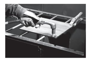
2. Press the torch's trigger to start the arc. Pause at the edge until the arc has cut completely through the workpiece.
