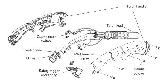
The entire hand torch and lead assembly can be replaced, or individual component parts can be replaced. Part numbers starting with 059 indicate complete torch and lead assemblies.
