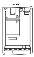
4. Pull the filter bowl straight down to remove.
