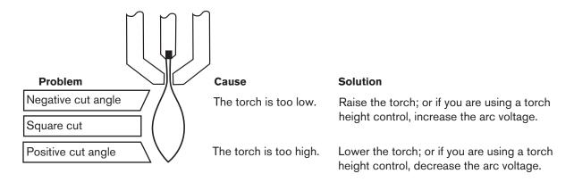
Note: The squarest cut angle will be on the *right* side with respect to the forward motion of the torch. The left side will always have some degree of bevel.
