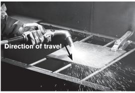
3. Pull the torch back and stretch the arc to 1-1/4 inch (32 mm). Push the plasma arc in the direction of the gouge you want to create. Increase standoff to create a shallower and wider gouge.
