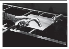
2. Fire the torch while still at an angle to the workpiece. Slowly rotate the torch to a perpendicular (90°) position.
