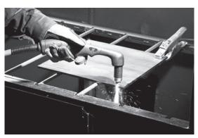
3. Drag the torch tip lightly across the workpiece to proceed with the cut. Maintain a steady, even pace.
