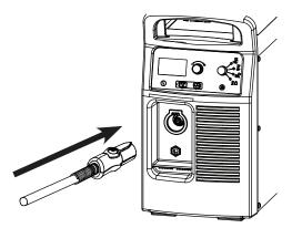
To remove the torch, press the red button on the connector and pull the connector out of the receptacle.
