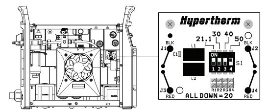
4. Set the DIP switches to one of the following settings and replace the power supply cover.
