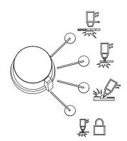
For cutting expanded metal, grates, metal containing holes, or any job that requires a continuous pilot arc. Using this mode to cut standard metal plate reduces consumable life.
