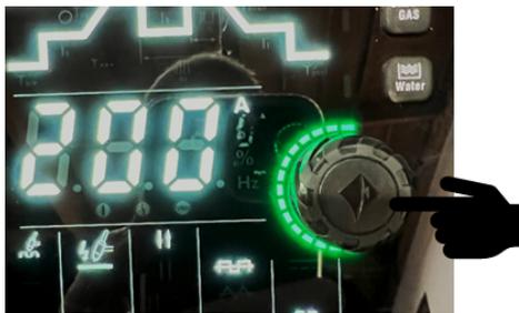
4. Adjust the Welding amperage dial on the front of the machine. This dial has a green background light indicating the amperage range. Turning clockwise will increase your amperage whilst turning anti-clockwise will decrease your amperage. Set your desired Max Peak Amperage then press the Amperage dial, that will lock in the set Base/Peak amperages. The relevant amperage icons will stop flashing.
