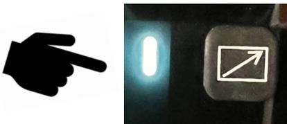
Remote control indicator light is on, the machine is in remote
