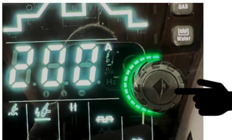
4. Adjust the Welding amperage dial on the front of the machine. This dial has a green background light indicating the amperage range. Turning clockwise will increase your amperage whilst turning anti-clockwise will decrease your amperage. To set your base amps and Peak amps navigate to the symbols and simply press the Welding amperage dial in. The icons will stop flashing.
