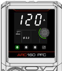
After selecting the electrode diameter the system will automatically select the welding current, Hot start current, and Arc force. Users can rotate the adjuster knob according to the welding requirements to fine-tune the welding current parameters.
