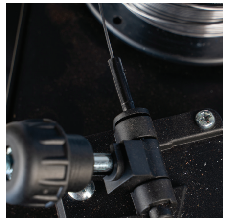
(6) Feed wire over the drive roller into the outlet guide tube, Push the wire through approx 6 Inches
