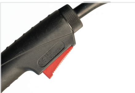
(7) Press and hold the Torch Trigger to feed the wire down the torch cable through to the torch head.
