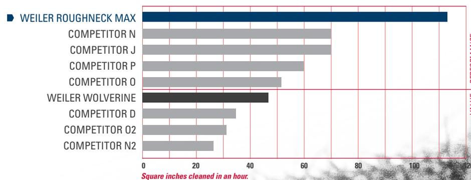
■ **Test Procedure:** Automated test on diamond plate, coated with powder metal. Test performed with a 4 1/2" 11amp grinder.
