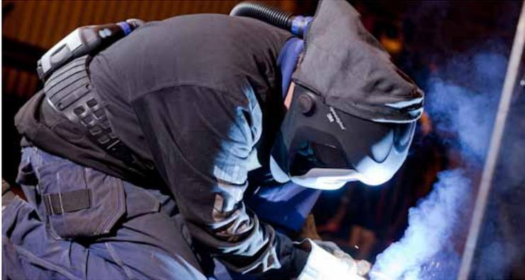
**Extended protection:** A flame-resistant headcover (used in this application) and ear/neck protection are available as accessories to all Speedglas 9100 series welding helmets.
