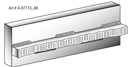
Figure 4-27: Staggered Intermittent Welding
