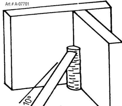
Figure 4-15: Single Run Vertical Fillet Weld
