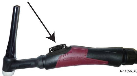
NOTE: The additional switches/controls below are interchangeable with the installed control in the TIG torch.
