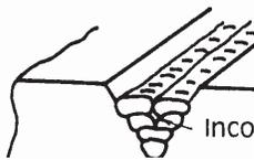
Figure 1 - Example of insufficient gap or incorrect sequence
