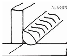
Figure 3: Example of Slag Inclusion
