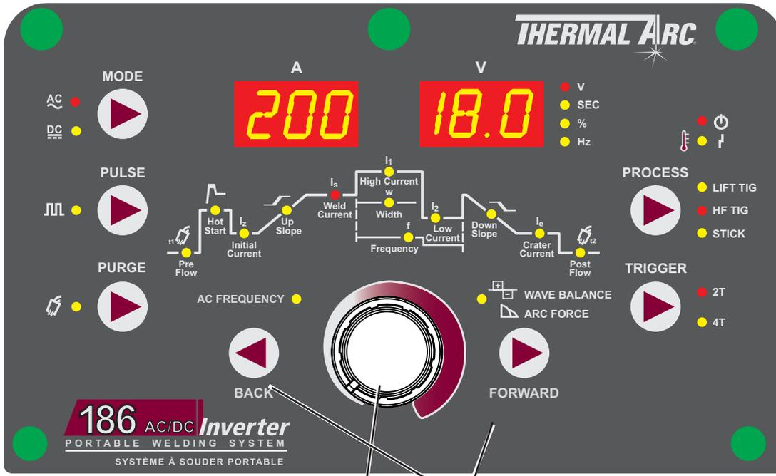
Adjust programming parameter using the Multi Function Control knob
