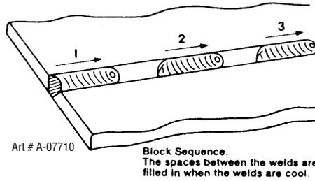
Figure 4-34: Welding Sequence
