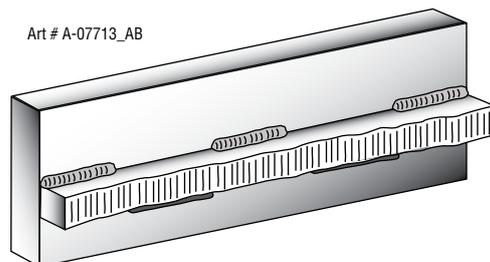
Figure 4-37: Staggered Intermittent Welding
