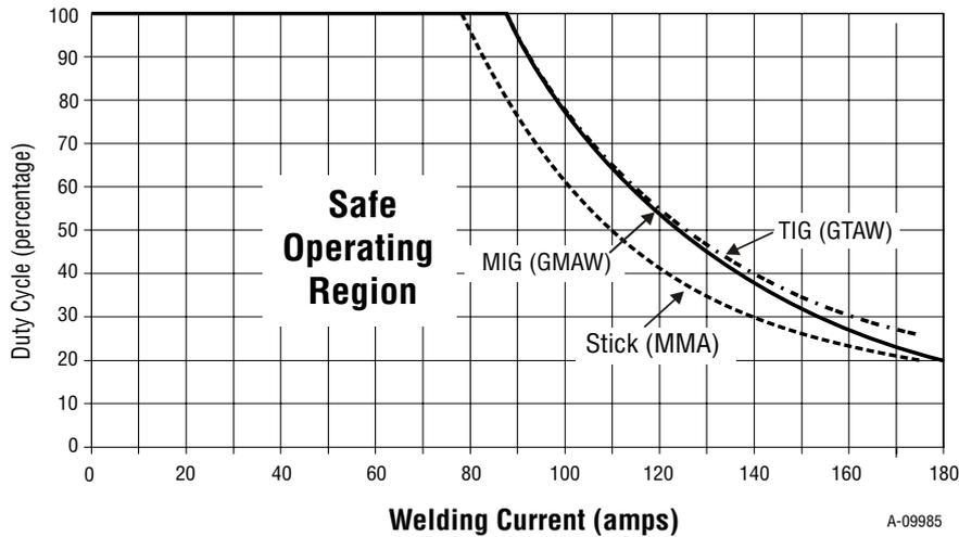
Figure 2-1: Fabricator 181i Duty Cycle
