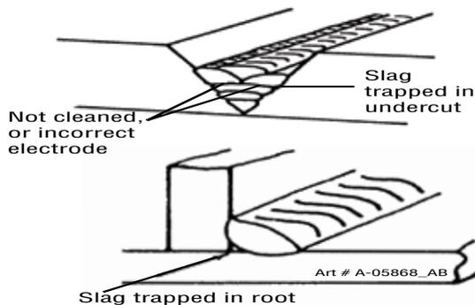
Figure 3: Example of Slag Inclusion
