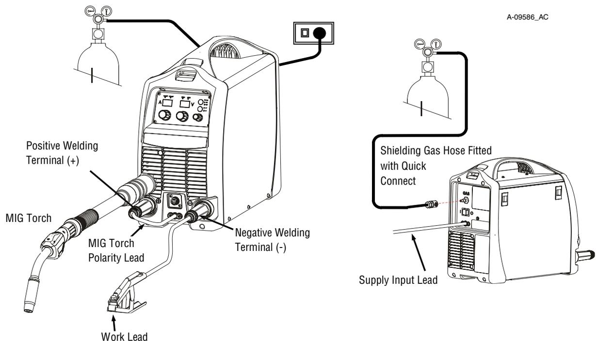
Figure 3-14: Setup for MIG Welding with Gas Shielded MIG Wire
