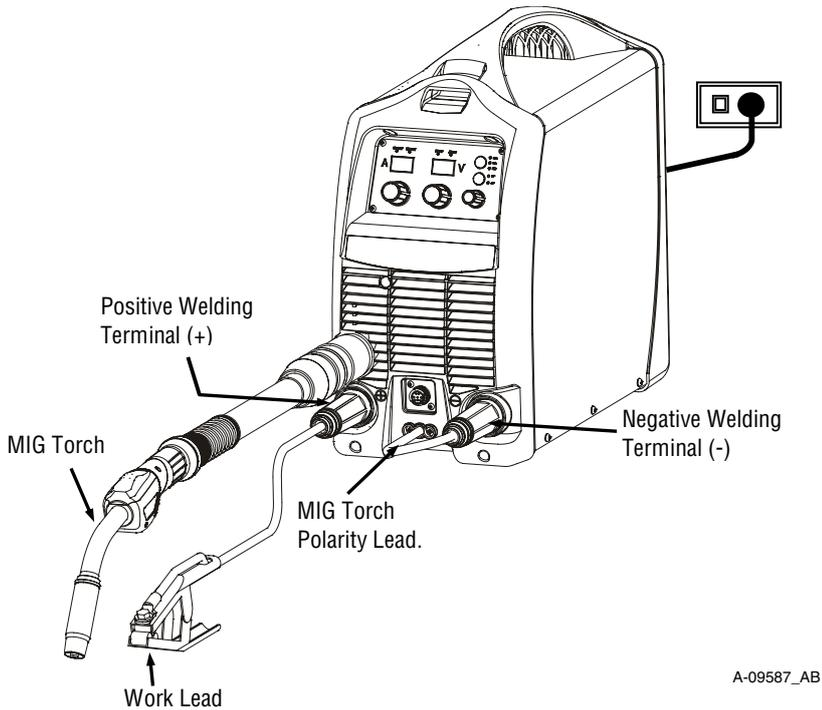
Figure 3-15: Setup for MIG Welding with Gasless MIG Wire
