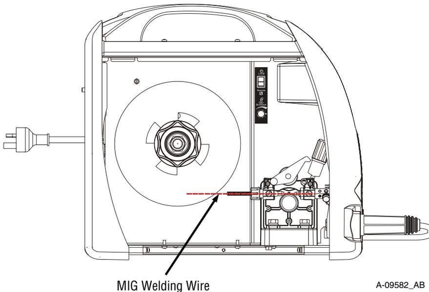
Figure 3-9: MIG Welding Wire - Installation
