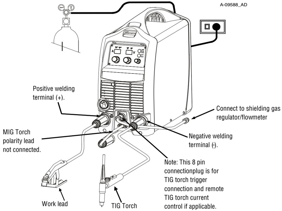
Figure 3-16: Setup for TIG Welding
