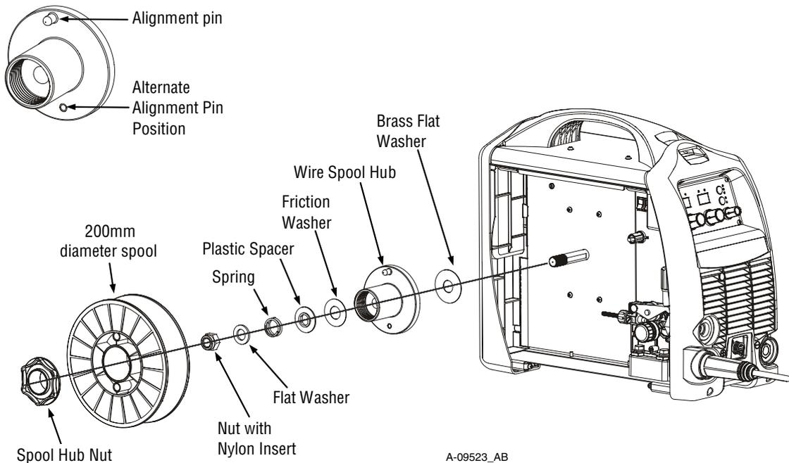
Figure 3-7: 200mm Diameter Spool Installation
