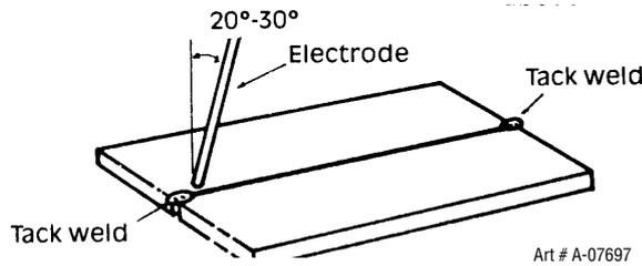
Figure 4-21: Butt Weld
