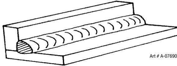
Figure 4-14: Horizontal-Vertical (HV) Position
