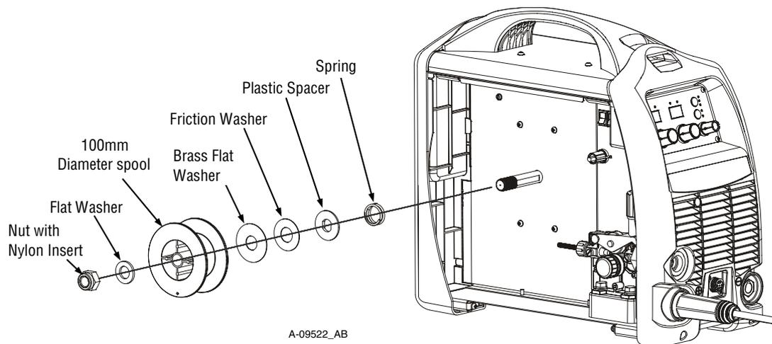
Figure 3-6: 100mm Diameter Spool Installation
